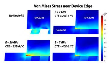
Figure 37: Von Mises (peak shear stress) in the edge-most solder bar under a temperature cycle change of  $\Delta T = +100$ C. Four different underfill conditions are simulated, with changing Youngs modulus (E) of the underfill and different CTE as well. Note that deformation has been exaggerated by the same scale in each picture.
