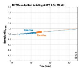
Figure 14: Comparison of inductive versus resistive hard switching on an EPC2204 FET switching at 80 V, 200 kHz. The same part was tested under inductive mode for the first four hours, followed by resistive mode for the next four hours. Both modes are essentially indistinguishable in terms of dynamic  $R_{DS(on)}$ .
