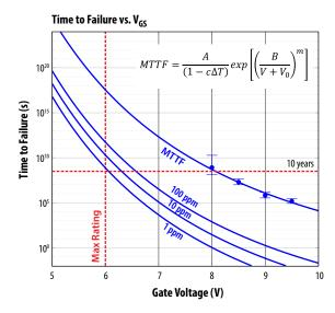
Figure 4: EPC2212 MTTF vs. V<sub>GS</sub> at 25°C MTTF (and error bars) are shown for four different voltage legs. The solid line corresponds to the impact ionization lifetime model. Extrapolations of time to failure for 100 ppm, 10 ppm, and 1 ppm are shown as well.
