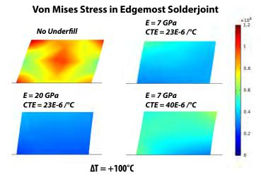
Figure 36: Von Mises (peak shear stress) in the edge-most solder bar under a temperature cycle change of  $\Delta T = +100$ C. Four different underfill conditions are simulated, with changing Youngs modulus (E) of the underfill, and different CTE as well. Note that mechanical deformation has been exaggerated by 20x in all cases.
