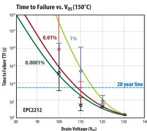
Figure 7: The data in Figure 4, as well as similar data taken at different temperatures, is translated into predictions of failure rates over time, temperature, and voltage.
