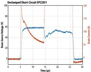
Figure 22: Fault under load test waveforms for a typical EPC2203 (top) and EPC2051 (bottom) at  $V_{DS}$  = 60 V,  $V_{GS}$  = 6 V and a 25  $\mu s$  drain pulse. The abrupt rise in drain current marks the time of catastrophic thermal failure.
