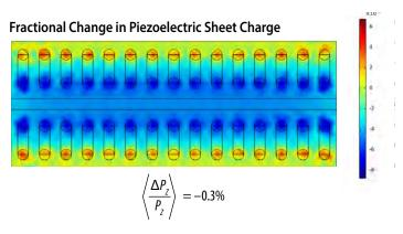
Figure 30: Fractional change in piezoelectric sheet charge for an EPC2206 under strain from 4 mm board deflection. The area averaged change in piezoelectric charge is less than -0.3%, while the peak change is around 0.8% in the immediate vicinity of solder bars. These changes in piezoelectric polarization are too small to create observable changes in device parameters  $V_{TH}$  or  $R_{DS(nn)}$ .
