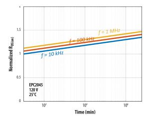
Figure B4: Modeled  $R_{DS(on)}$  vs. Time at three different switching frequencies, covering two orders of magnitude. Note that the effect of frequency change is a small vertical offset in the growth characteristic. The same offset would occur at different switch currents.
