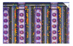
Figure 8: A magnified image of an EPC2212 eGaN FET showing light emission in the 1–2 μm wavelength range (SWIR) that is consistent with hot electrons. The SWIR emission (red-orange) has been overlaid on a regular (visible wavelength) microscope image.
