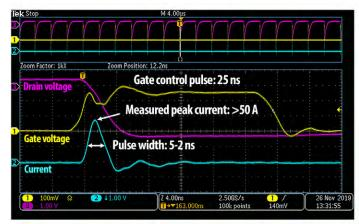
Figure C3: Typical lidar mode pulse waveforms.
