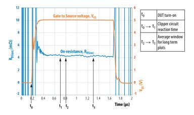
Figure 13: High time resolution oscilloscope waveform of the  $R_{DS(on)}$  in the first 1–2  $\mu$ s after a switch on transition. This waveform was taken on an EPC2218 after 1000 hours of continuous resistive hard-switching. Note that there is no evidence of the "fast dynamic  $R_{DS(on)}$ " recovery seen in other GaN technologies.
