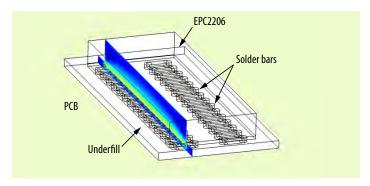
Figure 35: Simulation deck for finite element analysis of stresses inside EPC2206 under temp cycling stress. Die with underfill sitting on 1.6 mm FR4 PCB. Stress is analyzed along cut line shown.
