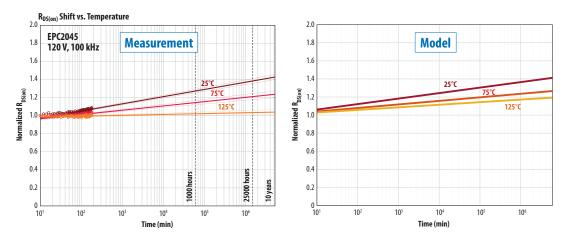
Figure 18: Comparison of measurement and model of dynamic  $R_{DS(on)}$  at various temperatures on EPC2045 at 120 V and 100 kHz.
