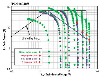
Figure 20: SOA results for EPC2045, EPC2212, EPC2014C. Measurements for 1 ms (purple triangles) and 100  $\mu$ s (green dots) pulses are shown together. Failures are denoted by red triangles (1 ms) or red dot (100  $\mu$ s). Note that for all parts, all failures occur outside the data sheet SOA region.
