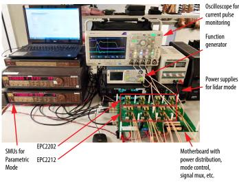
Figure C1: Lidar reliability test system
