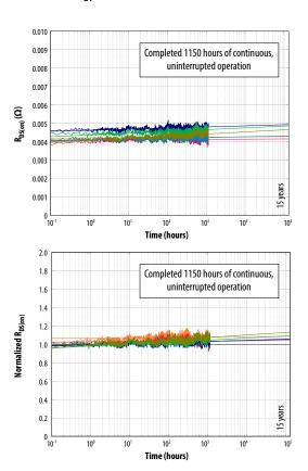
Figure 11: Long-term dynamic  $R_{DS(on)}$  for six samples of EPC2218 eGaN FETs under continuous resistive hard-switching operation for over 1000 hours at ambient temperature and a bias of 100 V. The graph on the top shows  $R_{DS(on)}$  versus Time, while the bottom graph shows  $R_{DS(on)}$  normalized to its value after the first 10 minutes. Note that even over 1000 hours of operation,  $R_{DS(on)}$  does not deviate from a simple log(time) growth dependence.
