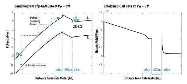
Figure A2: (Left) Band-diagram of eGaN gate under high forward bias (9 V). Far left corresponds to the gate metal; AlGaN front barrier is seen toward the right. Note that electron-hole pair production is depicted in the high field region near the gate metal. (Right): Electric field in the gate for the same conditions. Note the field is not uniform, reaching a peak > 2 MV/cm
