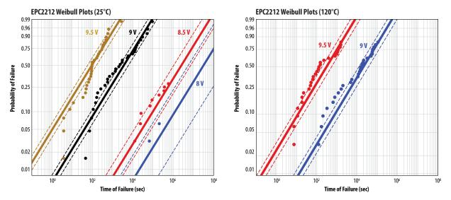
Figure 1: Weibull plots of gate-to-source failures of EPC2212. Note that very few failures occur even at 8  $V_{GS}$ , yet the device has a maximum  $V_{GS}$  rating of 6 V. The data on the top is at 25°C and the data on the bottom is at 120°C.
