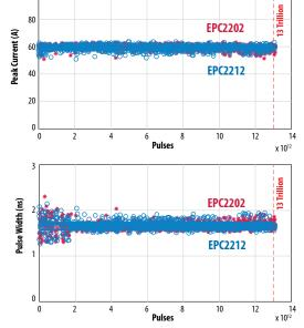
Figure 24: Long-term stability of pulse with (bottom right) and pulse height (top right) over 4.2 trillion lidar pulses. Data for four EPC2202 (red) devices and four EPC2212 (blue) devices are overlaid in the plots. Note the excellent stability of these key parameters over total number of pulses corresponding to a typical automotive lifetime. Oscilloscope image of pulses in upper left.
