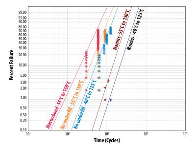
Figure 33: Weibull plots of Temperature Cycling results of EPC2206
