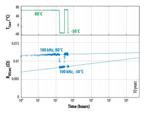
Figure 16: Effect of alternating hot-cold conditions on dynamic  $R_{DS(on)}$  for an EPC2059. (Top) Case temperature versus Time, as controlled by a thermoelectric cooler. (Bottom)  $R_{DS(on)}$  versus Time. Switching is continuous throughout at 100 V and 100 kHz.
