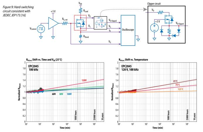
Figure 10: The  $R_{DS(on)}$  of a fifth-generation EPC2045 eGaN FET over time at various voltage stress levels and temperatures. On the left, the devices were tested at 25°C at voltages from 60 V to 120 V. The graph on the right shows the evolution of  $R_{DS(on)}$  at 120 V at various temperatures.
