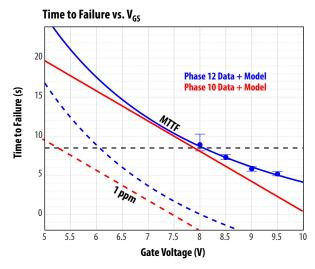
Figure A4: Comparison of: (red) Original gate acceleration data and simple exponential acceleration fit with (blue): Recent gate acceleration data along with impact ionization model fit. Dashed lines correspond to 1 ppm projections for each case.
