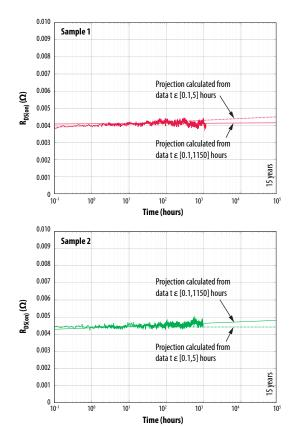
Figure 12: Comparison of log(time) fits to the  $R_{DS(on)}$  data, where the dashed line represents the fit over the first 5 hours, while the solid line represent the fit over the full 1150 hours. Data for two samples of EPC2218 are shown. Note that the short-term fit has a similar projection to the long-term fit, with small random differences of  $\pm$  10% on the 15 year projection.
