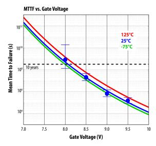
Figure 5: Measured MTTF for EPC2212 (25°C) measured at four different gate biases. Blue line is lifetime model. Red and green lines are predictions of the lifetime model at 125°C and −75°C respectively.
