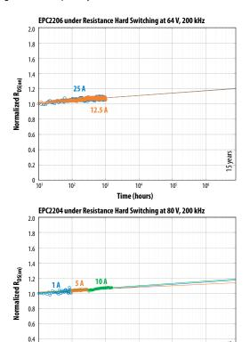
Figure 15: Effect of switch current on dynamic  $R_{DS(on)}$ . (top) Two EPC2206 devices were tested under resistive hard switching at 64 V, 200 kHz. (bottom) The same device was tested under inductive hard switching and three different currents at 80 V, 200 kHz. No discernible difference was found in the slope or intercept of the log(t) growth characteristics.
