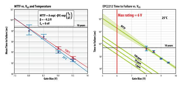
Figure 2: On the left is the mean time to failure (MTTF) for EPC2212 eGaN FETs versus  $V_{GS}$  at both 25°C and 120°C. On the right is a graph that shows the various probabilities of failure versus  $V_{GS}$  at 25°C.
